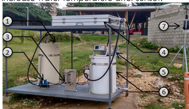
Figure 3. Experimental bank: 1. Water reservoir, 2. Pump, 3. Rotameter, 4. Solar collector, 5. Data acquisition unit, 6. Water reception tank, 7. Weather station.
