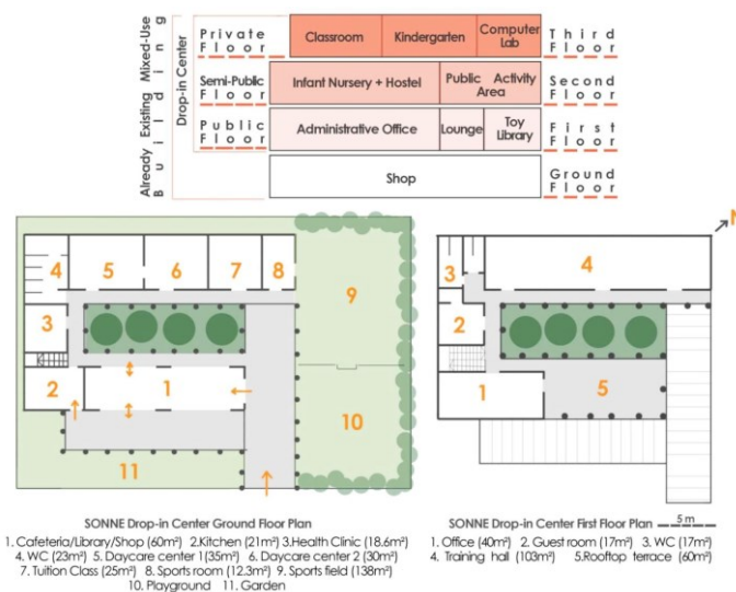
Figure 2. Top: Sectional zoning of Yayasan Chow kit drop-in center occupying 1st; 2nd; and 3rd floors (Developed by Authors based on Aliaas et al., 2012), Bottom: SONNE Street Children Center Design (Developed by Authors based on personal communication via email with SONNE Social Organization, 2018).
